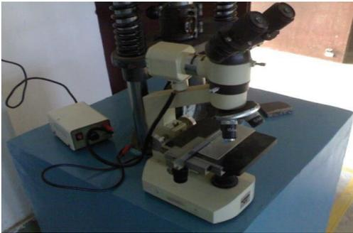
Fig. 2.17 Metallurgical Microscope
