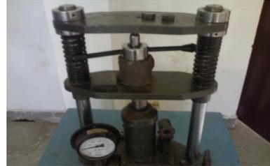
Fig.-2.11 Specimen mounting machine mounted specimen
