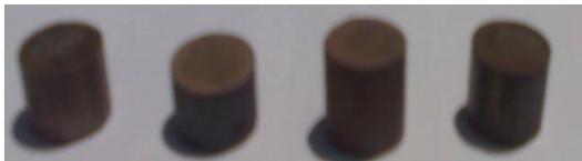
**Fig.2.5 Compacted billets of copper**
